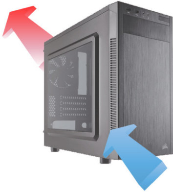
1| Exhaust fan: sucking warm air out of the chassis
